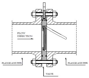
HORIZONTALLY ASSEMBLED VALVE ON VERTICAL PIPELINE WITH UPHILL FLOW
