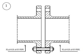
Insert one or two stud bolts and tighten them with nuts without forcing
