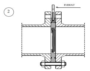
Holding the valve by the eyebolt, lower and set it on the already inserted stud bolt
