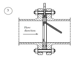
Insert the other stud bolts and tighten them with the nuts. Be sure that the valve's external diameter is equidistant from the screws and that the direction of the arrows on the external diameter is the same as the one of the flow
